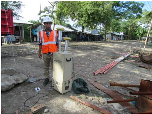
Ambient Air sampling at Construction Camp
