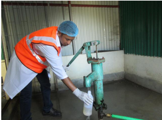
Ground Water collection at Project Area
